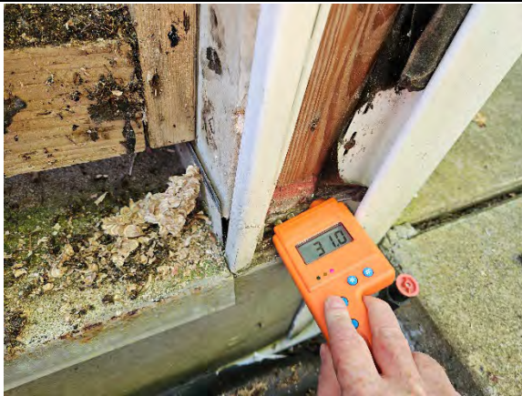
Photo 2.3: Wet reading (31.0) at framing.
