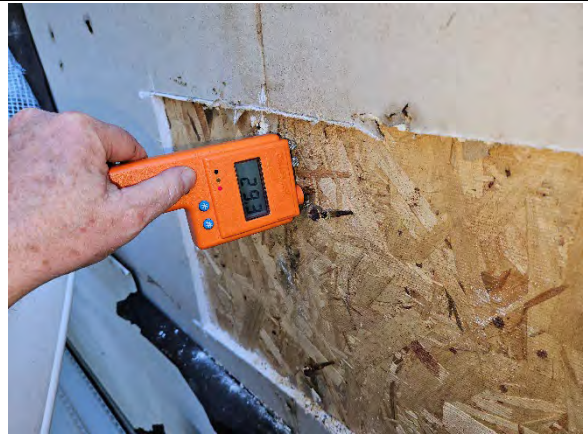
Photo 1.10: Wet reading (29.3) at OSB sheathing.
