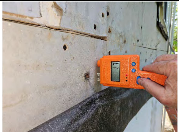
Photo 14.6: Wet reading (1.7) at gypsum sheathing.
