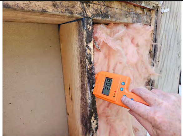
Photo 16.16: Wet reading (20.8) at framing.
