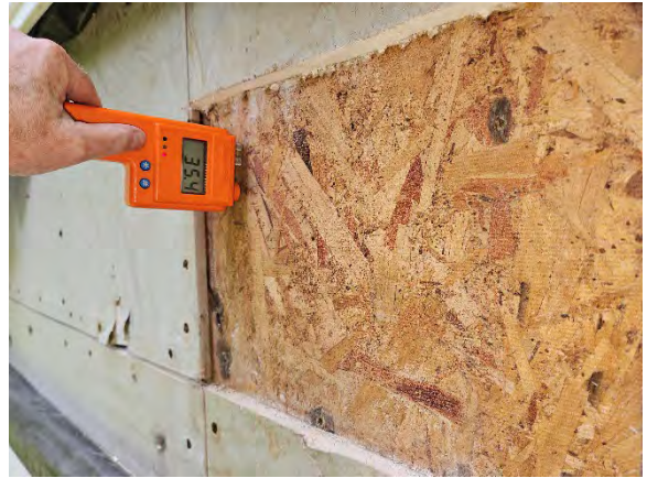
Photo 14.8: Wet reading (35.4) at OSB sheathing.
