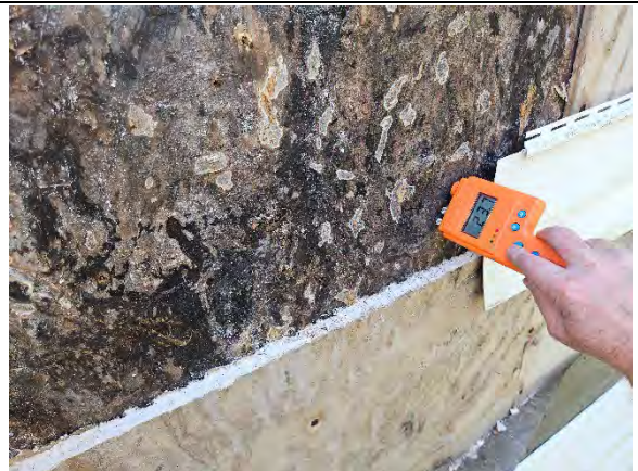
Photo 16.12: Wet reading (23.7) at OSB sheathing.
