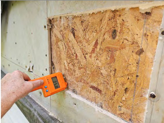
Photo 14.9: Wet reading (35.8) at OSB sheathing.
