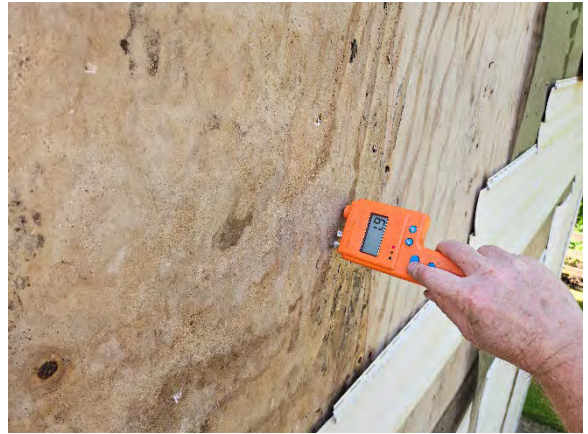
Photo 16.8: Wet reading (1.9) at gypsum sheathing.
