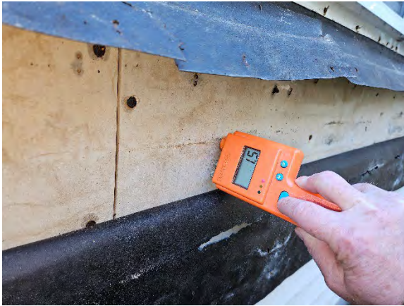
Photo 1.7: Wet reading (1.5) at gypsum sheathing.
