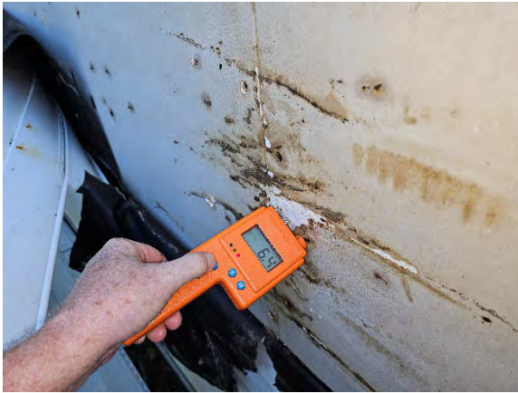
Photo 1.7: Wet reading (6.4) at gypsum sheathing.
