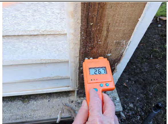
Photo 2.6: Wet reading (26.7) at deck column.
