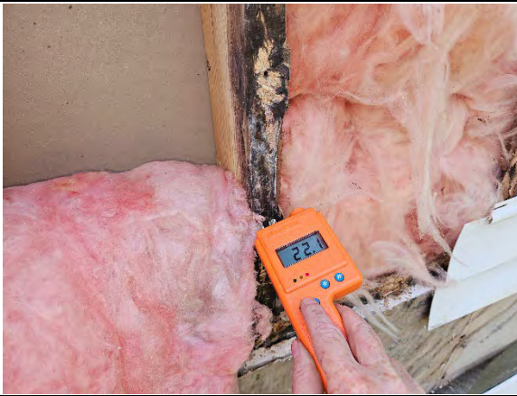
Photo 16.15: Wet reading (22.1) at framing.
