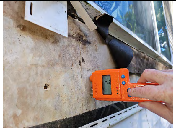
Photo 5.6: Wet reading (2.4) at gypsum sheathing.
