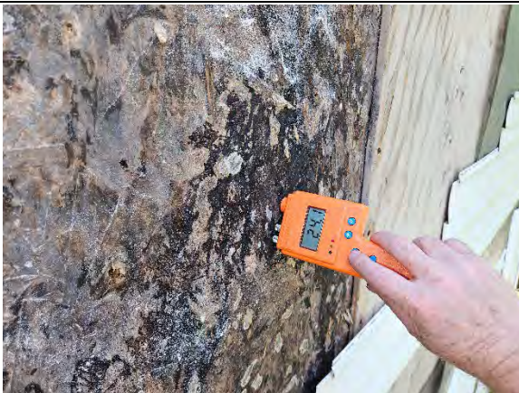
Photo 16.11: Wet reading (24.1) at OSB sheathing.
