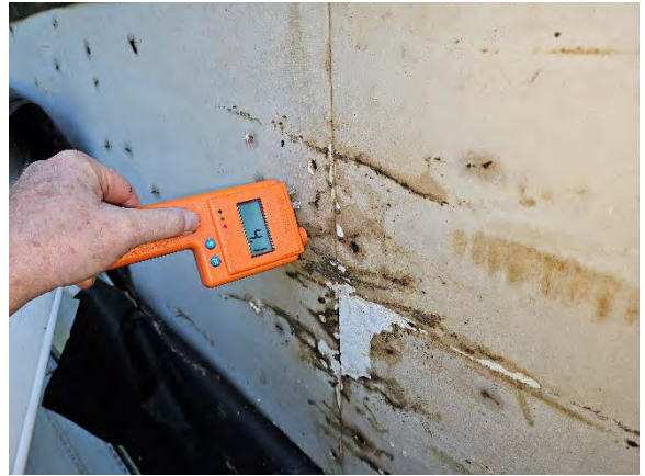
Photo 1.8: Wet reading (4.1) at gypsum sheathing.
