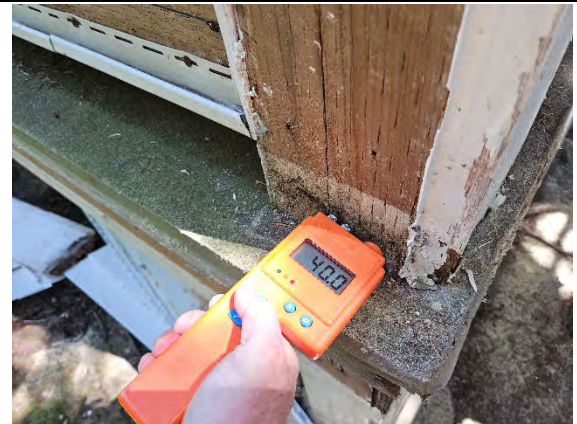
Photo 10.4: Maximum reading (40.0) at deck column.
