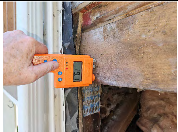
Photo 15.16: Wet reading (19.1) at framing.
