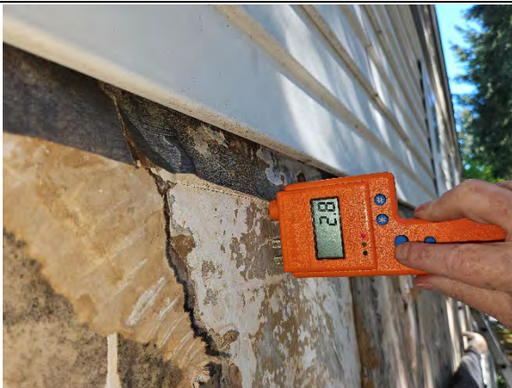
Photo 4.9: Wet reading (2.8) at gypsum sheathing.
