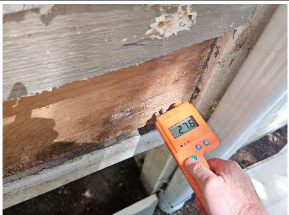
Photo 10.6: Wet reading (27.6) at deck framing.
