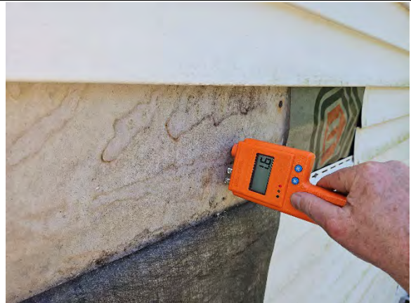
Photo 15.6: Wet reading (1.6) at gypsum sheathing.
