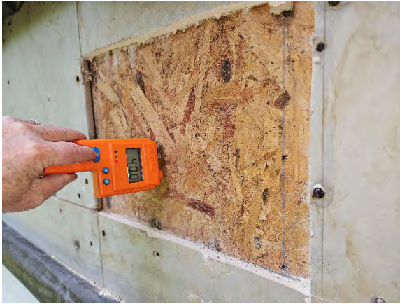
Photo 14.7: Maximum reading (40.0) at OSB sheathing.
