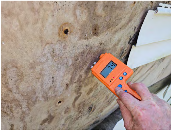
Photo 16.7: Wet reading (7.4) at gypsum sheathing.
