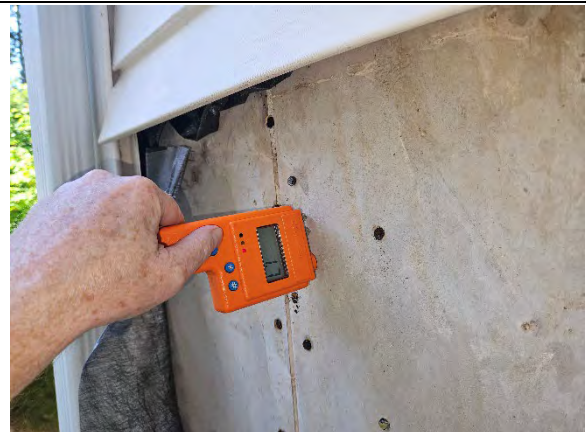
Photo 11.6: Wet reading (1.7) at gypsum sheathing.
