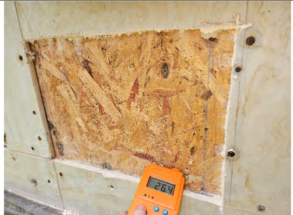
Photo 14.10: Wet reading (26.4) at OSB sheathing.
