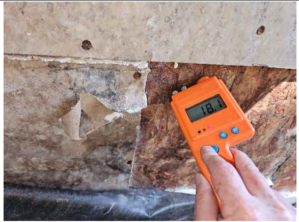
Photo 12.10: Wet reading (18.1) at OSB sheathing.
