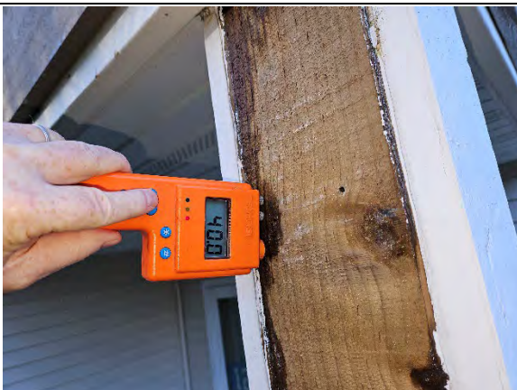
Photo 2.5: Maximum reading (40.0) at deck column.
