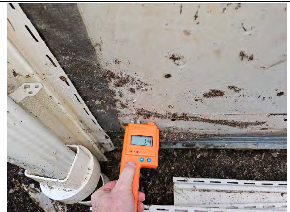
Photo 6.6: Wet reading (1.4) at gypsum sheathing.
