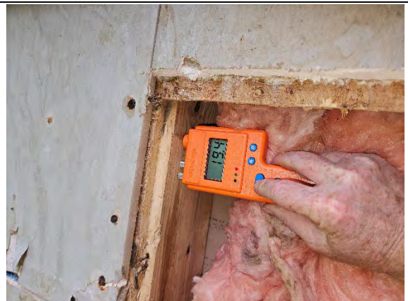
Photo 14.12: Wet reading (19.4) at framing.
