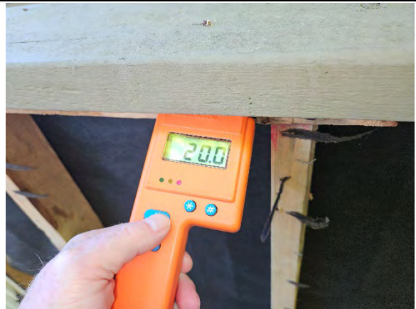
Photo 2.4: Wet reading (20.0) at framing.
