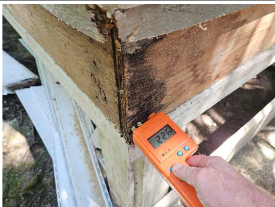
Photo 10.5: Wet reading (22.6) at deck framing.
