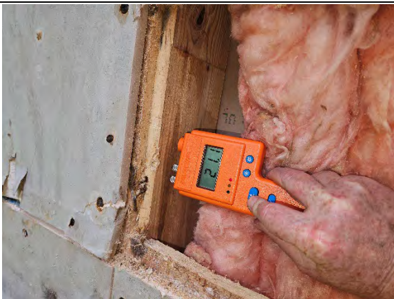
Photo 14.11: Wet reading (21.4) at framing.
