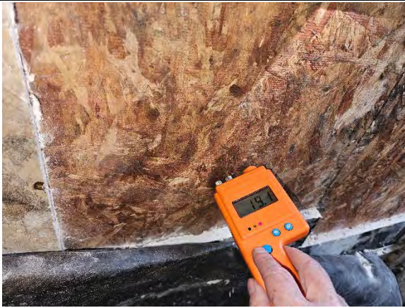
Photo 12.9: Wet reading (19.1) at OSB sheathing.
