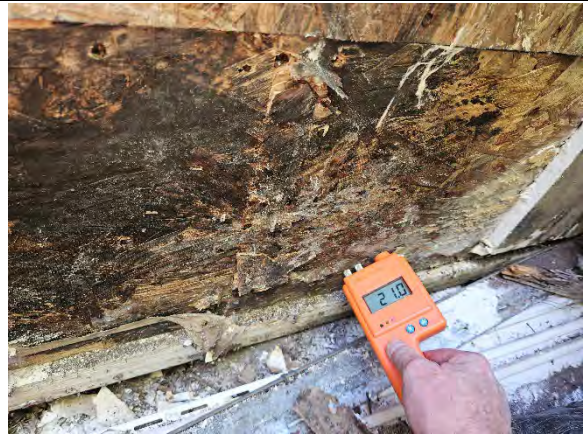
Photo 5.10: Wet reading (21.0) at OSB sheathing.
