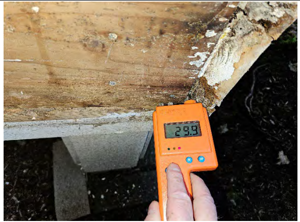
Photo 1.10: Wet reading (29.9) at deck framing.
