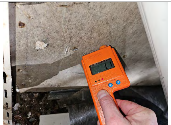
Photo 3.6: Wet reading (1.1) at gypsum sheathing.
