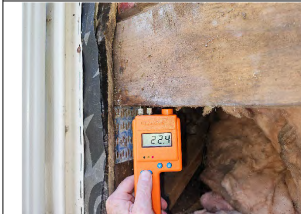
Photo 15.15: Wet reading (22.4) at framing.
