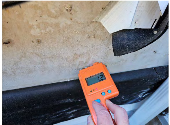
Photo 1.8: Wet reading (1..2) at gypsum sheathing.
