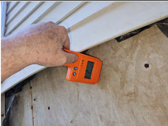
Photo 11.5: Wet reading (2.1) at gypsum sheathing.
